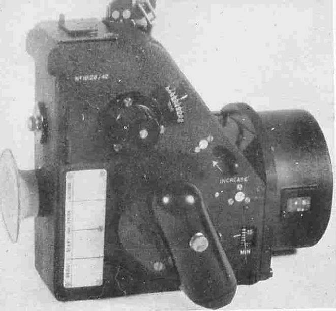
*The Mark IXa Sextant takes 60 shots at 2-second intervals and gives a final average reading over the two minutes of observation, thus reducing the accumulation of errors prevalent in a reading from a single shot.*
