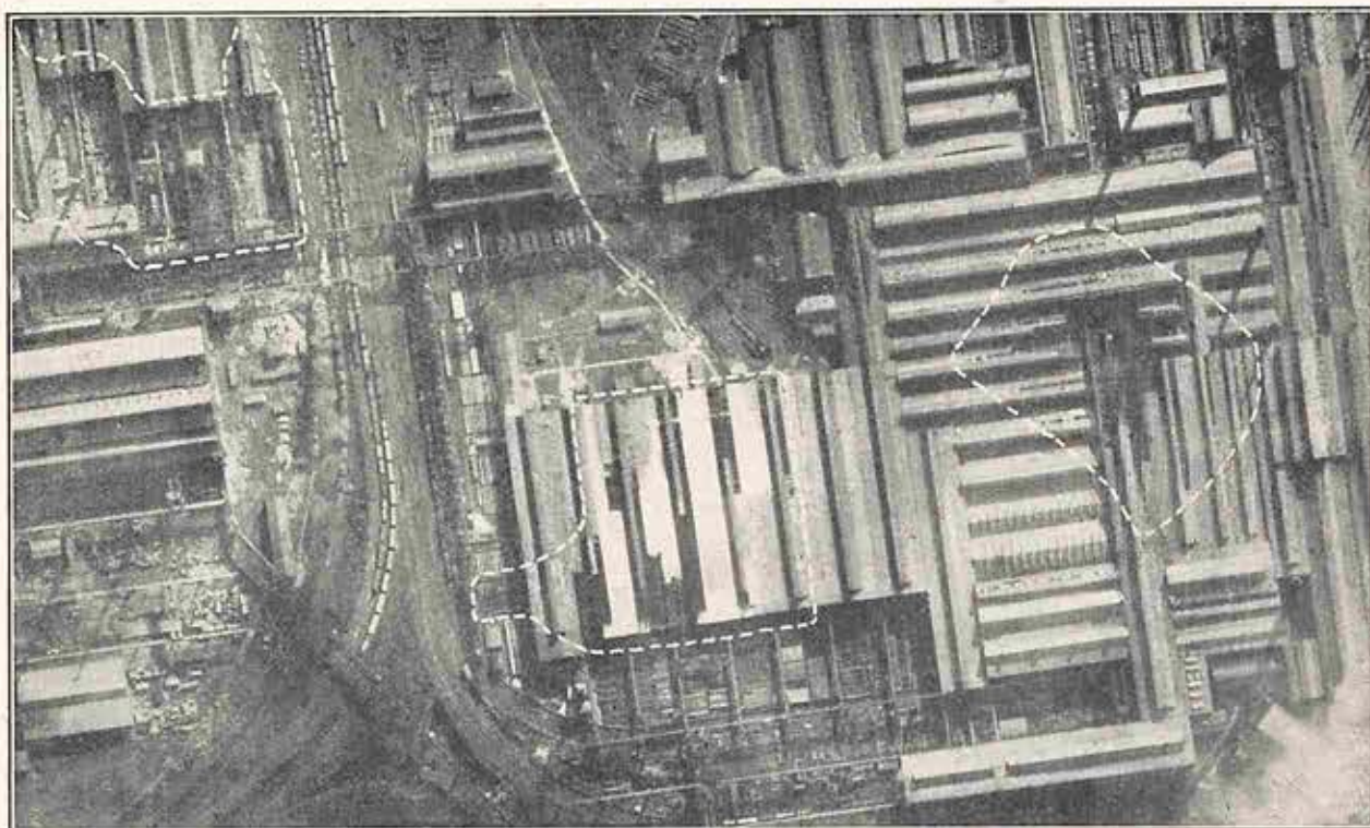
FIG. 1.—The Thyssen Works at Hamborn (one of the largest steelworks in the whole of Germany and Occupied Europe) was seriously damaged by high explosive bombs in July, 1942. A heavy bomb burst in the heart of the huge rolling mill (right), destroying 150,000 square feet of roofing and much of the supporting structure. Other damage is outlined in the above photograph, and the effects on the working of the plant are referred to on page 4.
