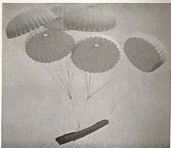
Parachutes opened completely and the boat has assumed correct bows down attitude. The fore and aft inflation chambers beginning to inflate.
