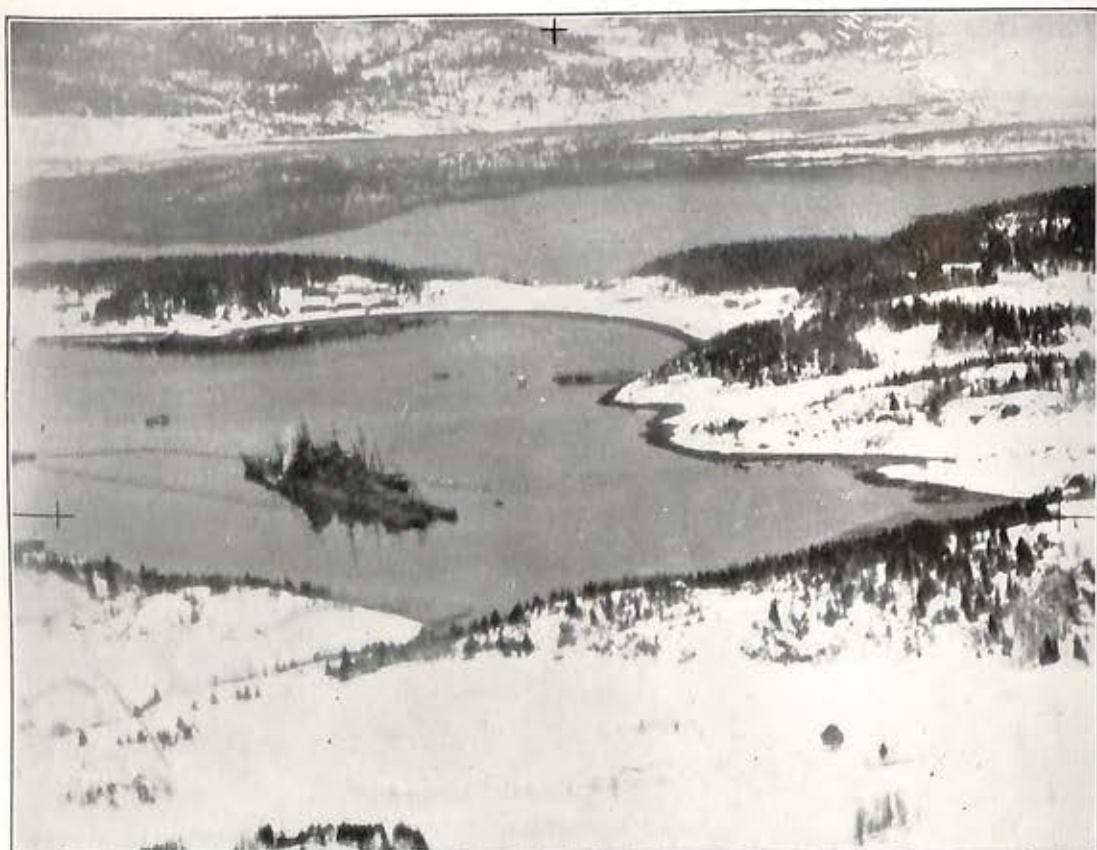
Prinz Eugen and Scheer in Lo Fjord. Photographs by P.R.U. taken on March 9, 1942. Double booms surround the warships. Scheer is only seen above, to left. A submarine supply ship lies alongside Eugen , and a floating crane at the stern is repairing damage; on its removal the stern was seen to have been cut square.
