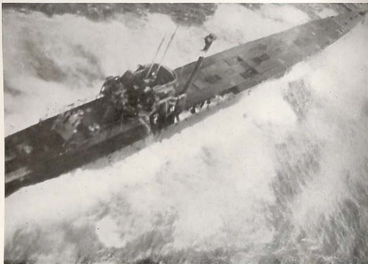
This type IXC (740-ton) U-Boat, U.1229, was sunk by aircraft from U.S.S. Bogue on August 20, 1944. After the first attack the U-Boat crash-dived and then raised her schnorkel in an attempt to proceed at schnorkel depth. When this was found to be impossible, the boat surfaced with her schnorkel and periscope still extended. It is to be noted that in this class of U-Boat the schnorkel is on the starboard side, whereas the 500-ton U-Boats have their schnorkels on the port side.
