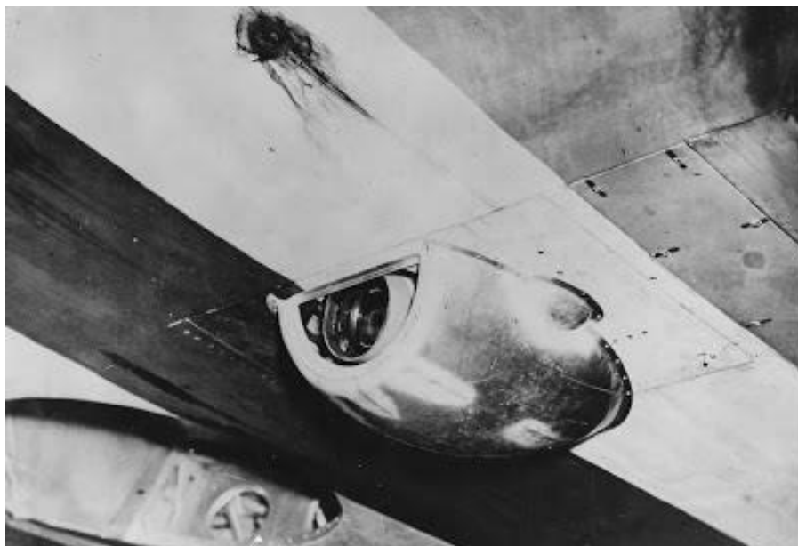
Wing-mounted forward-facing camera; note flak damage
