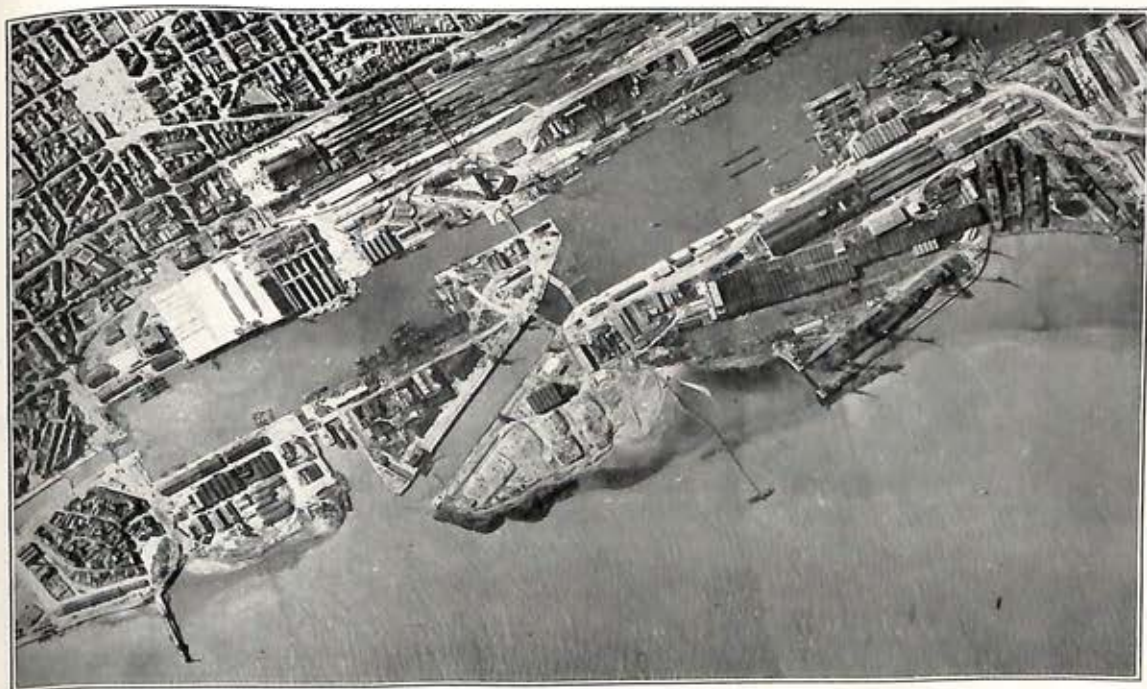
Plate 4. PHOTOGRAPHS BY P.R.U.: THE GROWTH OF THE U-BOAT PENS AT ST. NAZAIRE. Above, the site cleared, 4th April, 1941. Middle, three pens constructed, 26th May, 1941. Below, the completed pens, after the Commando raid, 7th April, 1942: the outer lock gate is clearly destroyed, and the inner is being strengthened by sand pumped from the harbour.
