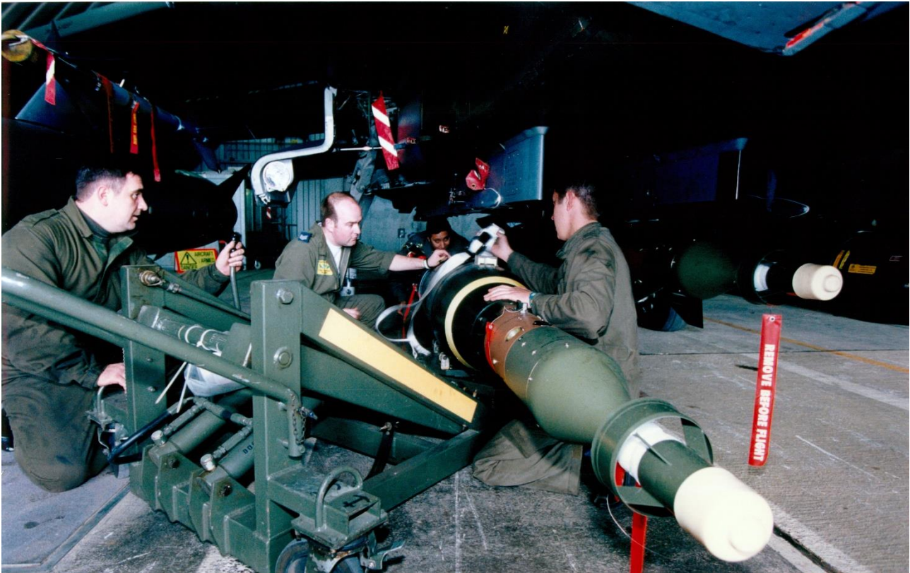
RAF armourers loading a Paveway II LGB on to a Tornado GR1 at RAF Bruggen during Allied Force.
