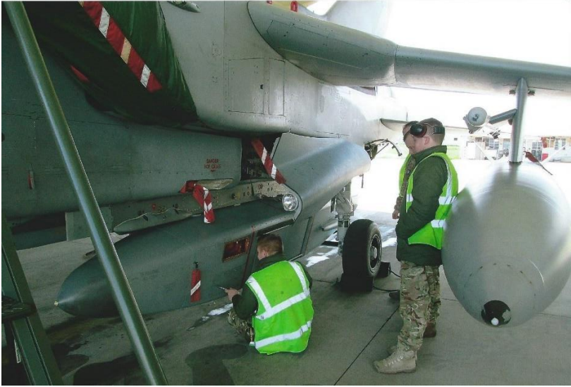
The Tornado GR4's RAPTOR reconnaissance pod being prepared for an Operation Shader mission in May 2015.
