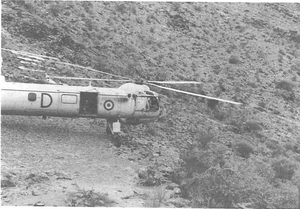
Re-supply in the Radfan 2 miles East of Thumier. Note the front wheels 'castored' to prevent movement down the slope.
