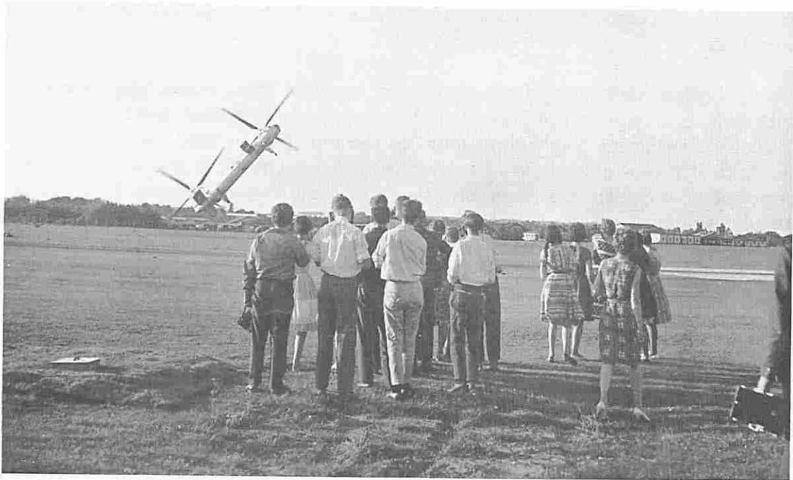
Last flight of the wooden-bladed full manual controlled pre-production Belvedere, just prior to the crash while rehearsing for the 1961 SBAC show at Farnborough. The Sycamore type rotor blades are clearly shown.
