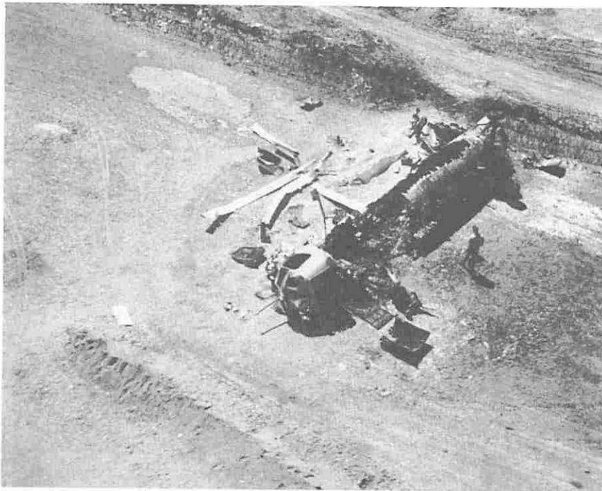
The result of loss of a nut retaining part of the Belvedere control linkage—Aden.
