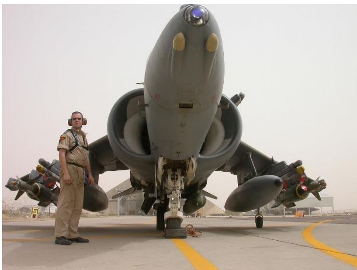
One of the all-important TIALD-capable GR7s; the pod is visible to the right of the fuselage.
