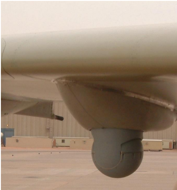
The MX-15 camera on a Nimrod MR2 during Telic.
