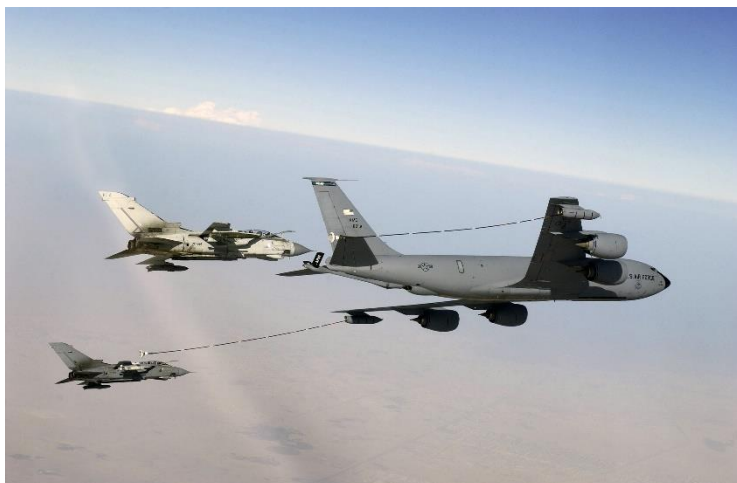
AAR was critically important in Telic: here, two RAF GR4s are refuelling from a USAF KC-135.
