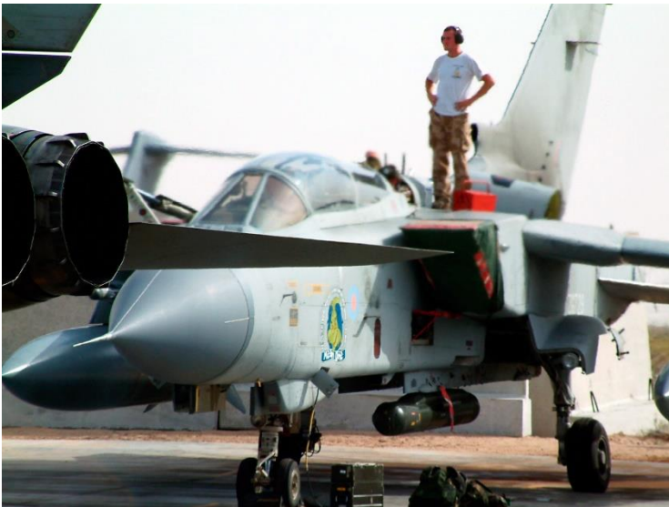
A Combat Air Wing GR4 with its TIALD pod on clear display; despite its limitations, TIALD was of critical importance to GR4 and GR7 operations.
