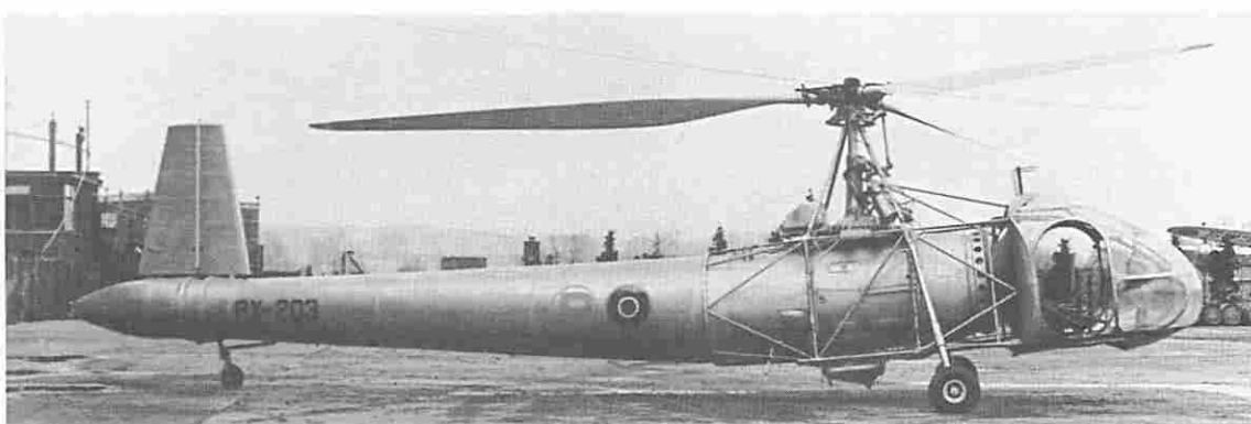
Cierva W9 (1947), one of the series of experimental helicopters by Weir.
