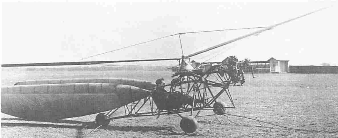
Mr Raoul Hafner flying (tethered) his R-2 helicopter—being the second experimental machine he designed and built in Vienna, and the one he brought back with him when he came to England in 1933—Heston airport.
