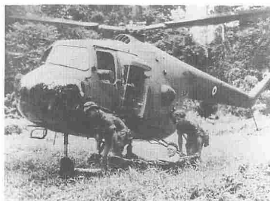
The Mk 14 sycamore could carry 2 stretchers athwartships (but rarely used the upper stowage). A stretcher was sometimes not available and had to be manufactured 'on the spot'. The passenger doors enlarged in the Mk 14 to facilitate stretcher carriage are clearly shown.
