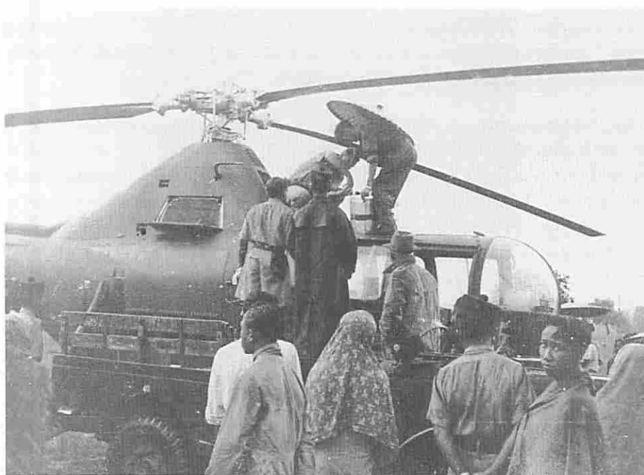
Re-fuelling a Dragonfly in the rain from an air dropped 'flimsy' petrol can in Malaya. The fuel had to be poured through a special filter.
