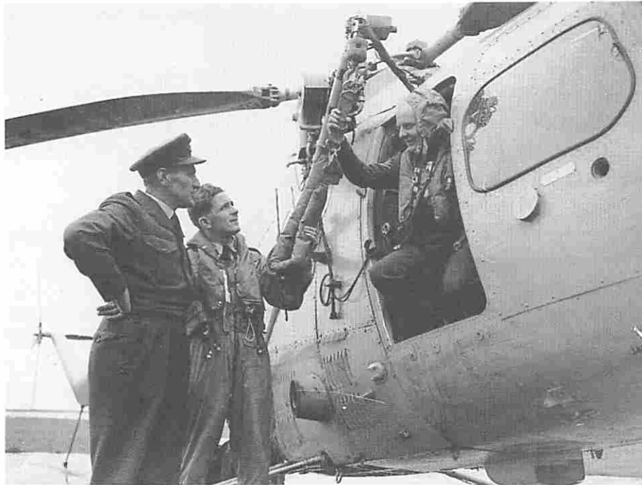
Winch fitted to Sycamore Mk 14.
