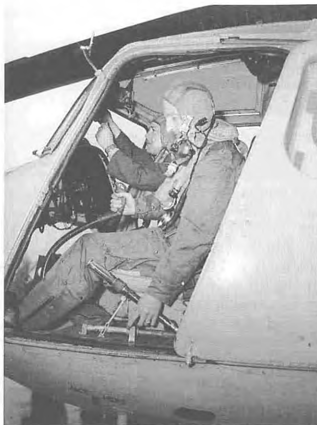
Sycamore Mk 13 showing the duplicated collective lever which was replaced by a single central collective lever in the Mk 14 production aircraft.
