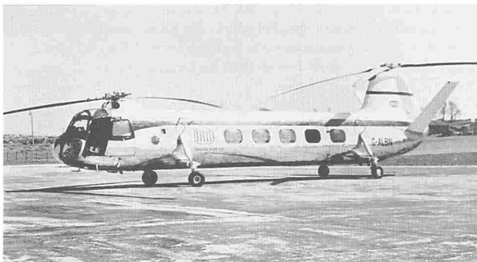
Prototype of the Bristol 113 (1954)—developed from the Sycamore and with Sycamore rotor blades (front rotor blades reversed) and powered by two Leonides piston engines, it was the forerunner of the Bristol 191 and 192 (the Belvedere).
