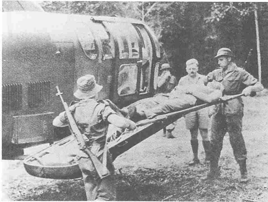
Initial handling trials in Malaya in 1950—the external pannier for the Dragonfly HC2 with a practice casualty.
