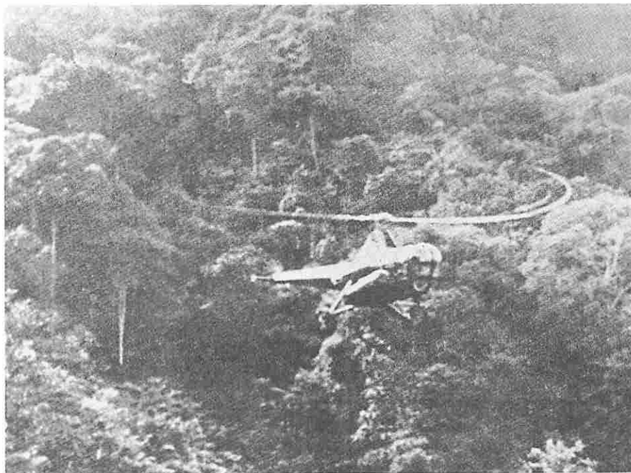
Initial handling trials in Malaya, 1950. The Dragonfly HC2 has a starboard external pannier fitted. The condensation in the tip vortex shows the high level of humidity.
