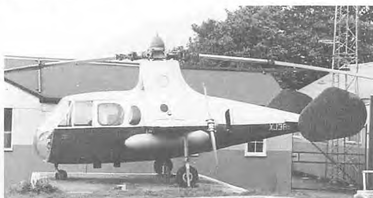
The Mk 2 Gyrodyne having two forward facing propellers. It was used experimentally only.
