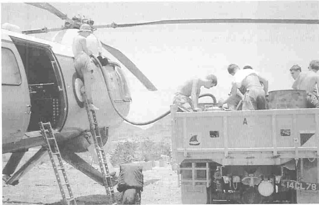
Belvedere refuelling at Thumier using 44 gallon drums and a mechanical pump. Note the proximity of the front engine jet pipers.
