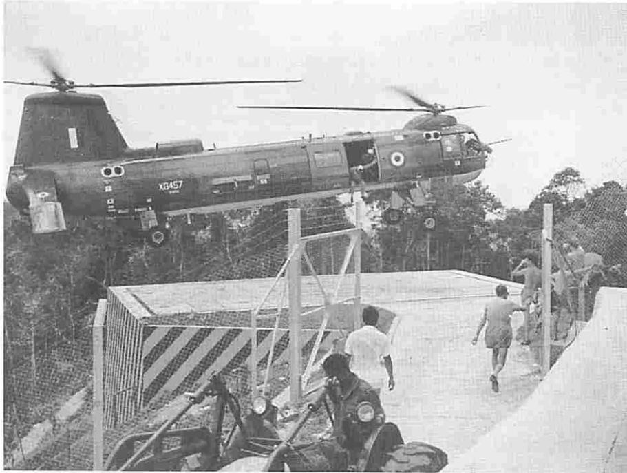
The Belvedere had a permanent LZ built for it on the top of Penang Hill in North Malaya, where the aircraft was used extensively to deliver components for the Ground Radars station being built there.
