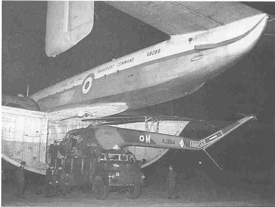
Unlike the Whirlwind, the Sycamore could be loaded into the Beverley without the need to interfere with the rotor hub and blades. This method of deployment was used as part of the immediate response to the Brunei revolt.
