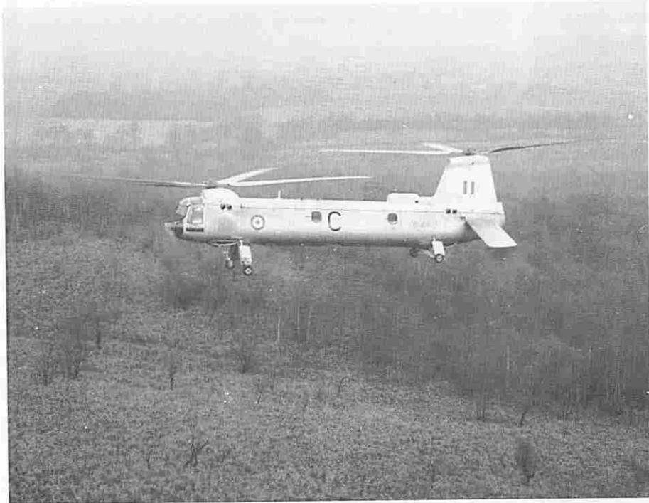
Pre-production Belvedere of the BTU near Odiham. Note the small wheels and large tail stabilisers—both modified in the later production aircraft.
