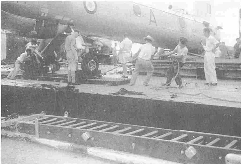
Manoeuvring a Belvedere on a supply ship deck prior to being lifted off by crane.
