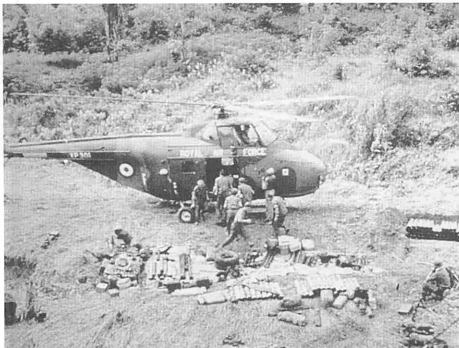
The Whirlwind Mk 10 could deliver the 105 mm gun and ammunition, but the gun had to be stripped to allow the load to be spread over several sorties.
