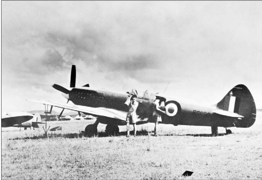
Indirect air action: two airmen remove the aerial cameras from a Spitfire PR 19 of 81 Squadron in Malaya in March 1954
