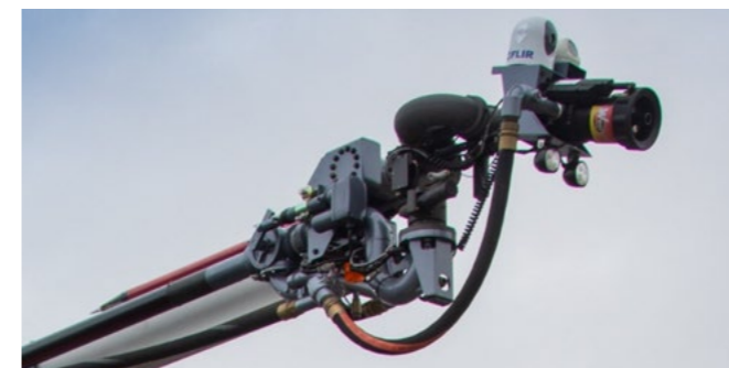
Oshkosh's Hydro-Chem Nozzle (HRET) Hydro-chem nozzle (HRET) – 1800L / 3600L per min (Max 3600L on 100% flow rate) Dry Powder (from hydro Chem nozzle) – 8kg per second
