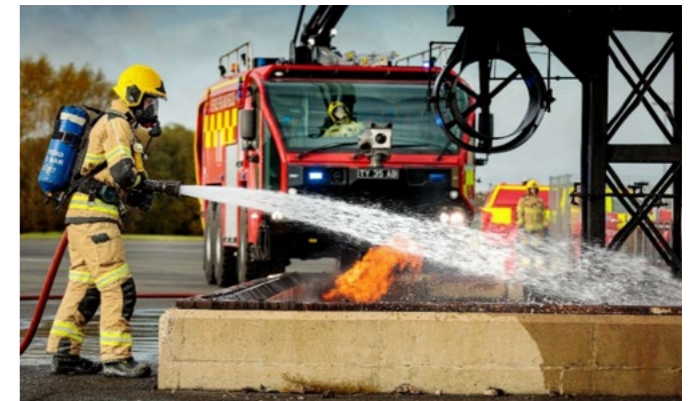
Firefighting Pump Capabilities The Oshkosh also has a Single Stage Centrifugal Pump that can produce up to 7511 litres per minute at 15.5 bar pressure
