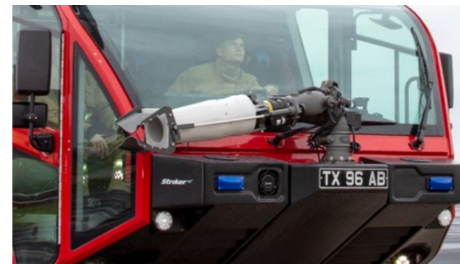
The Bumper Monitor Bumper Monitor - 3000L / 6000L per min (Max 6000L on 100% flow rate)
