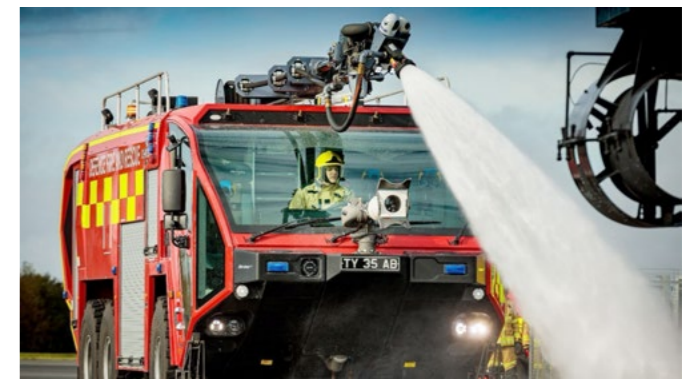
Hydro-Chem Nozzle in action
