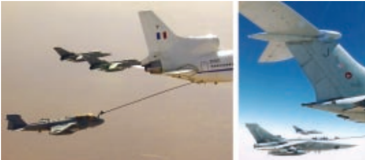
A Tristar refuels an American EA-6B Prowler while 2 Tornados await their turn (left), a Tornado F3 refuels from a VC10 (right)
