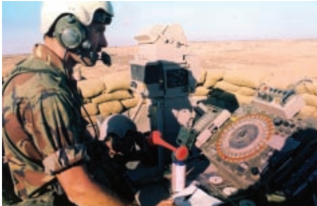
Rapier FSB1M fire control point
