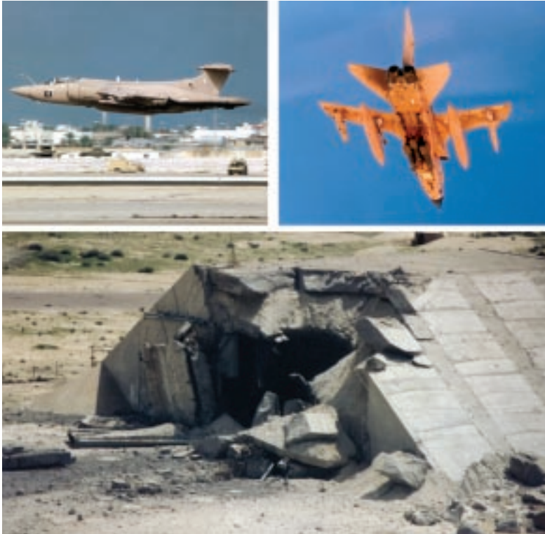
Pave Spike Buccaneer, Tornado GR1 with 3 LGBs, The result of an LGB attack against an Iraqi HAS
