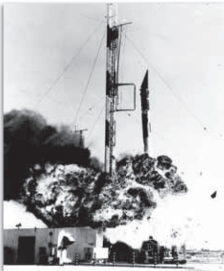
Test of Vanguard launch vehicle for U.S. International Geophysical Year (IGY) program to place satellite in Earth orbit. Malfunction in first stage caused vehicle to lose thrust after two seconds and vehicle was destroyed.
