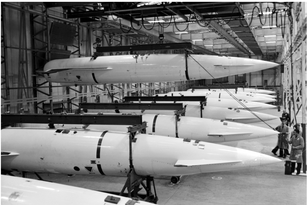
Blue Steel stand-off nuclear missiles in the storage hangar at Scampton, Lincolnshire, in February 1963. Blue Steel, built by Avro, was introduced into service by 617 Squadron in 1963. It carried a one megaton warhead and was used by two squadrons in Bomber Command - 617 (Avro Vulcan B2) and 139 (Handley Page Victor B2).
