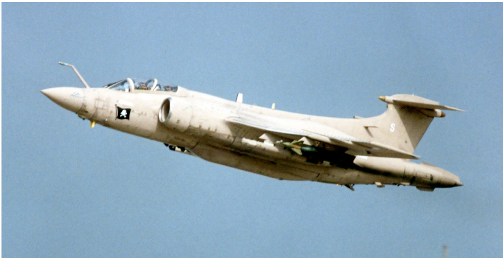
Operation GRANBY: A Buccaneer of 208 Squadron taking off from Muharraq, Bahrain, carrying a Paveway LGB and Pavespike targeting pod on the port wing weapons pylons.
