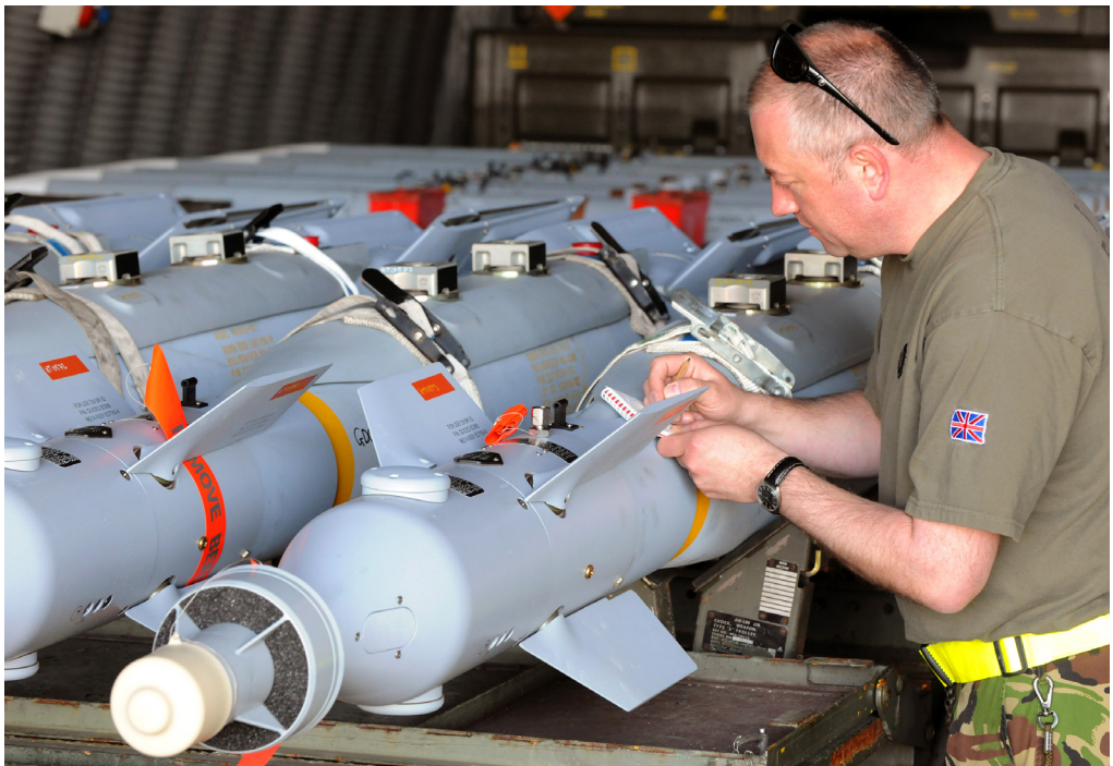
Armourers position and check Enhanced Paveway IV bombs prior to loading them onto aircraft taking part in Operation Ellamy.
