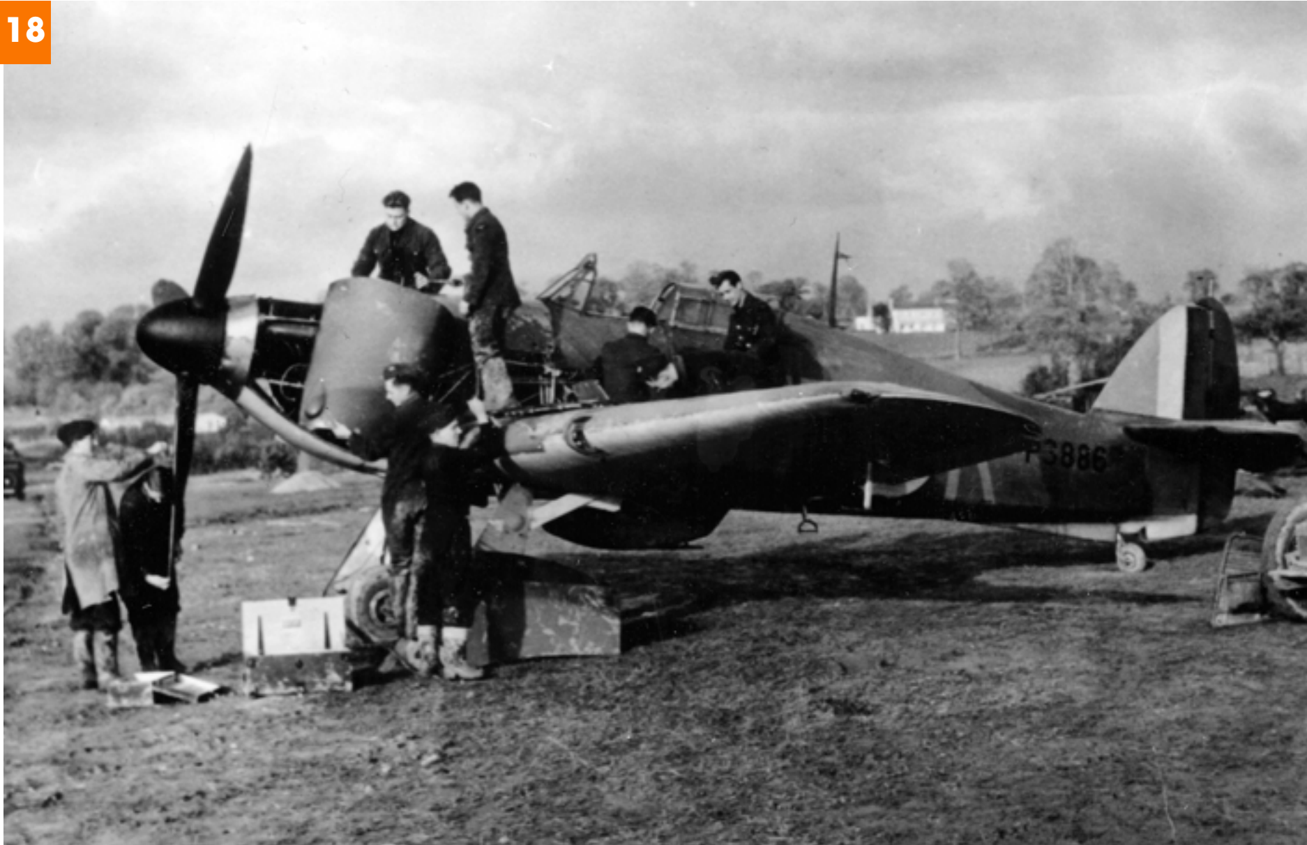
“Battle of Britain 1940 – Repairs underway by squadron engineering personnel to a Hurricane.” – One of the subsequent lessons drawn by Fighter Command was that the semi-autonomous maintenance system, introduced during the pre-war expansion of the RAF, was not that well matched, in size and flexibility, to the mobility demanded of the flying squadrons.
