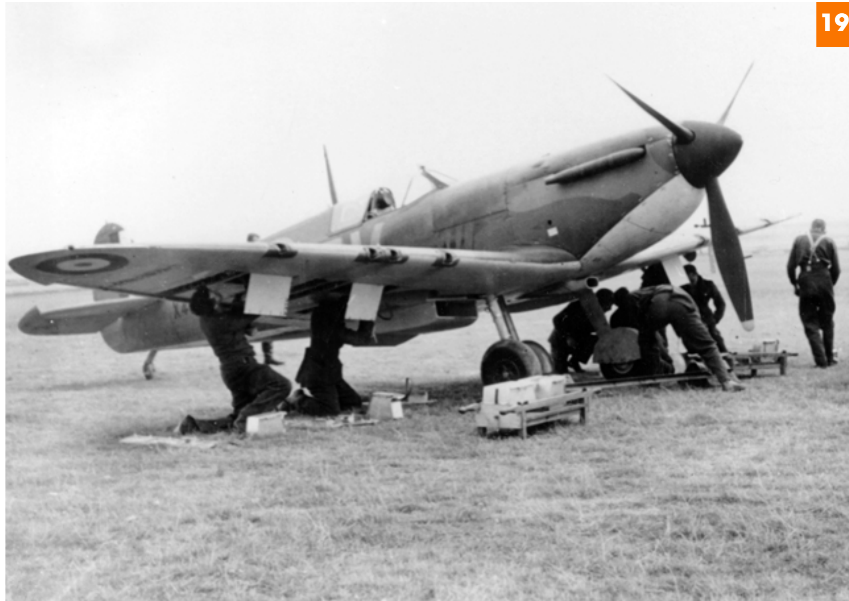
“Battle of Britain 1940 – A Spitfire is serviced and rearmed by squadron engineering personnel.” – At this stage of the war, maintenance was carried out on a semi-autonomous basis, but by 1942 a more efficient, and more mobile centralized system had been introduced.
