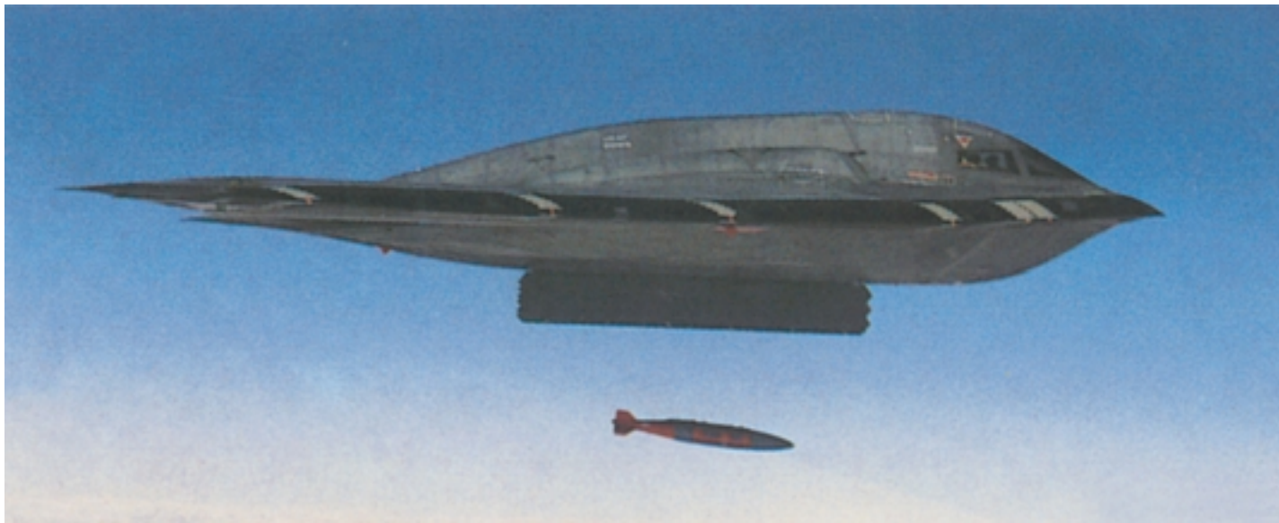
B-2s used JDAM weapons against infrastructure targets, some within Belgrade city limits. The GBU-31 JDAM (Joint Direct Attack Munition) is a 2,000 lb bomb with an optional penetrating warhead.
