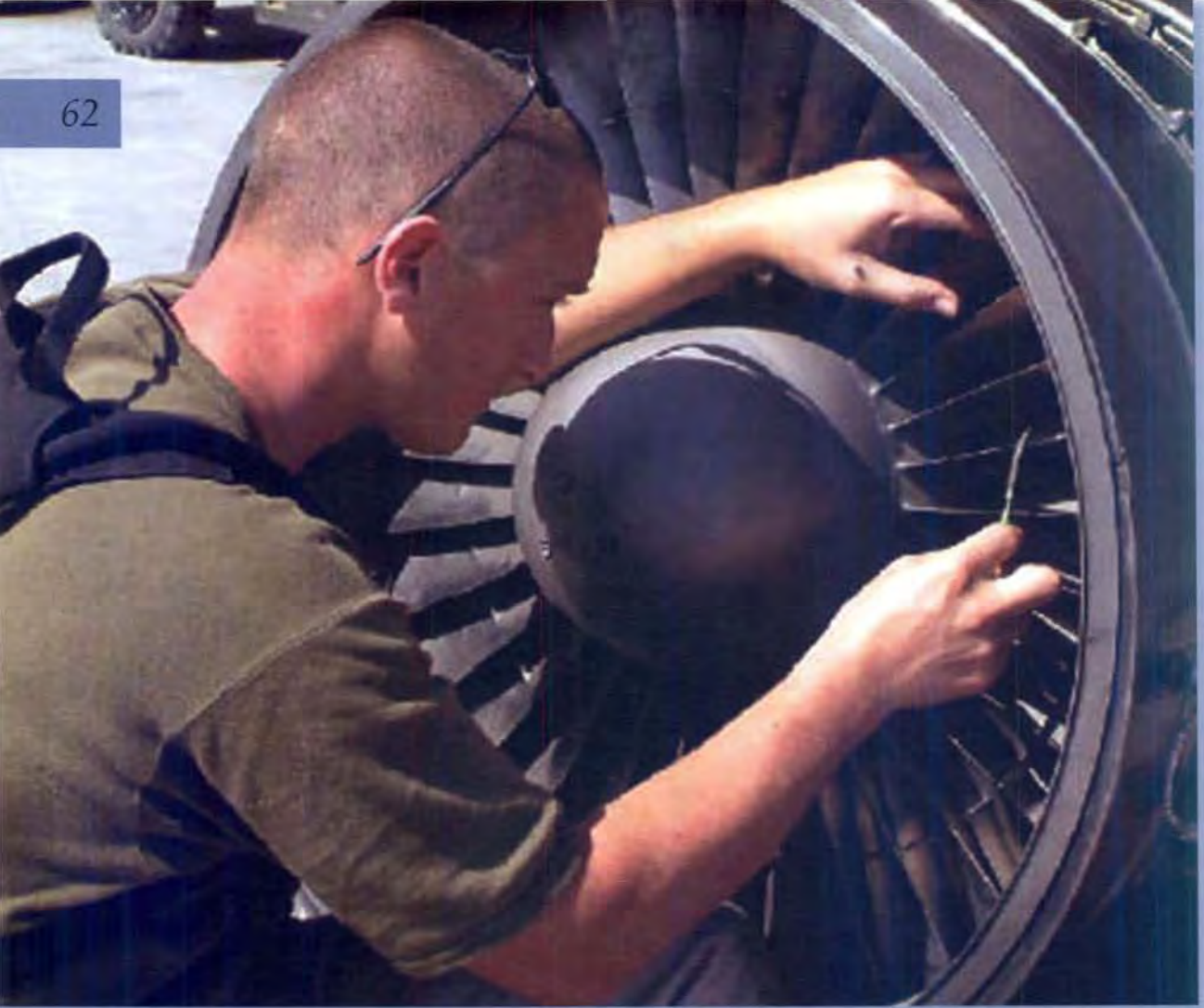
RAF ground crew repair a damaged engine compressor during Operation TELIC in 2003 Headquarters Strike Command Corporate Communications
