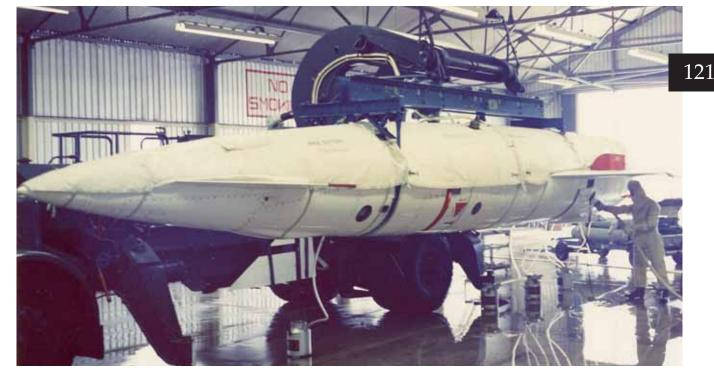
A Blue Steel missile being refuelled with high test peroxide (HTP), RAF Scampton
