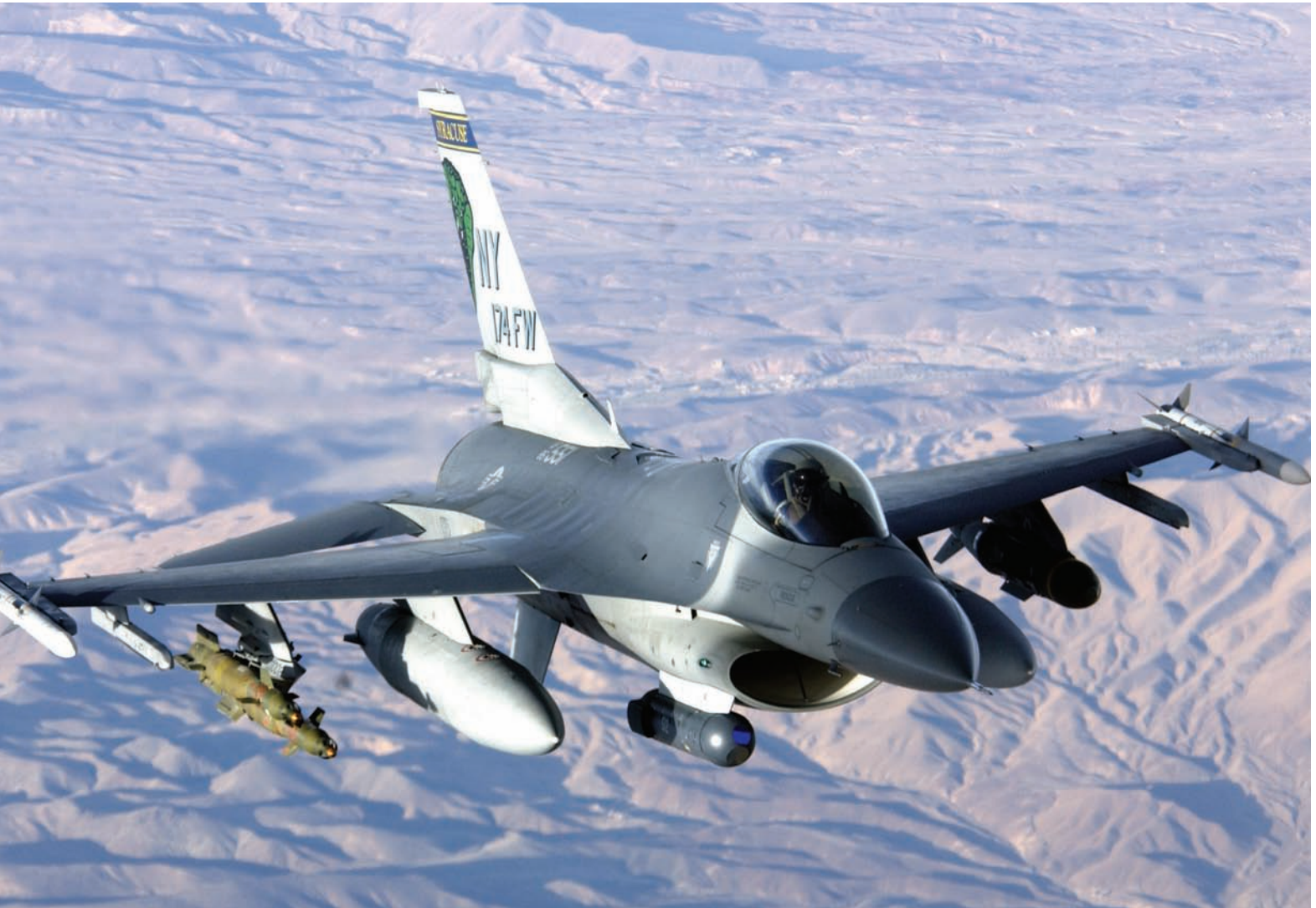
An F-16 over Afghanistan; note the LITENING targeting pod under the fuselage
