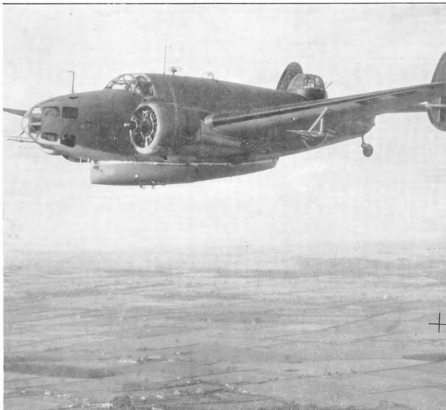
Air/Sea Rescue Hudson in flight, with an airborne lifeboat attached.
