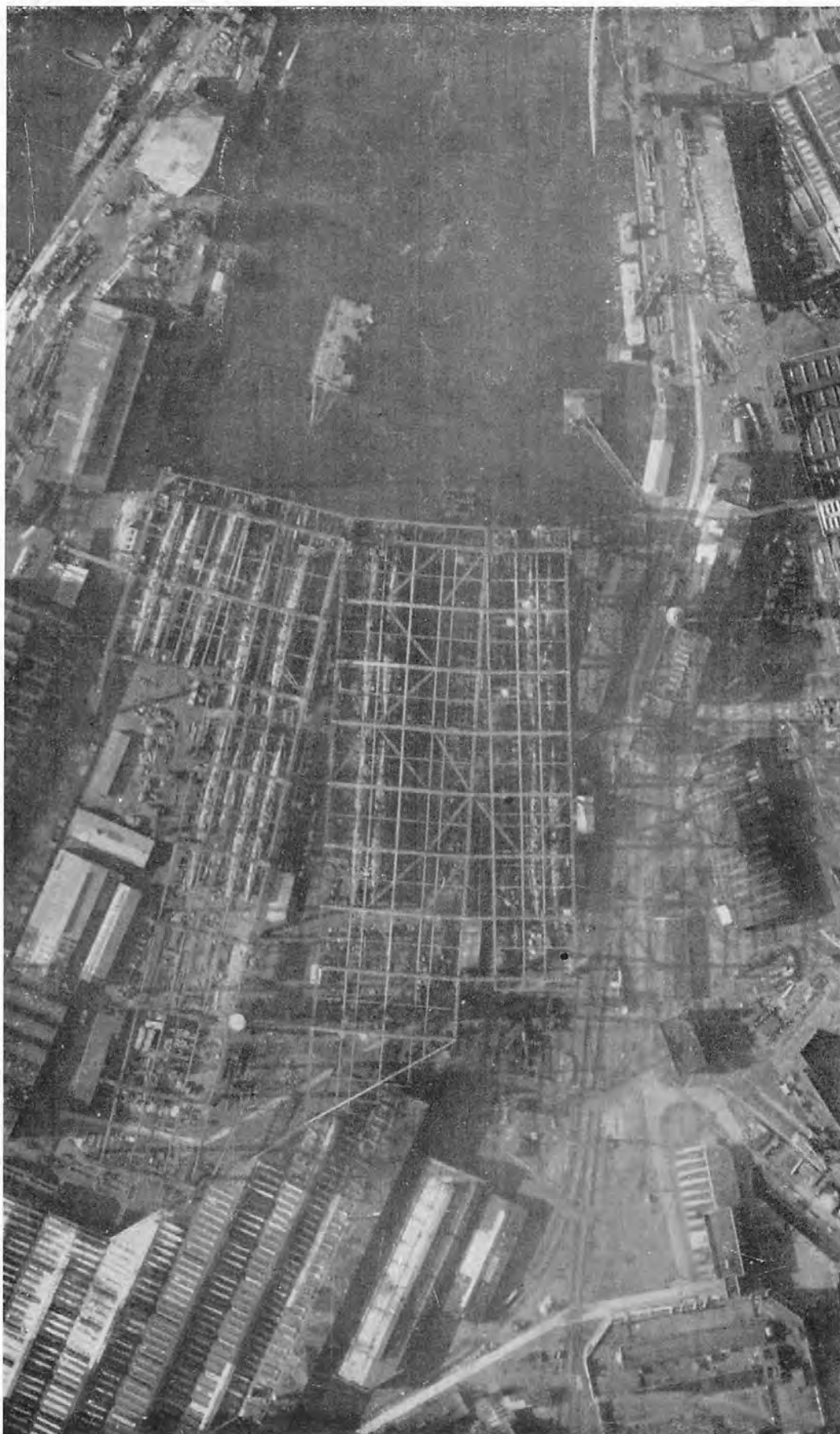
In previous numbers of the Review , reference has been made to the new type XXI U-Boats, which the enemy has been building for some time. These are assembled very quickly from prefabricated sections. Although the sections are made at a number of points there are only three assembly yards. The Blohm and Voss Yards at Hamburg, seen above, are one. A number of U-Boats can be clearly seen on the slips,
