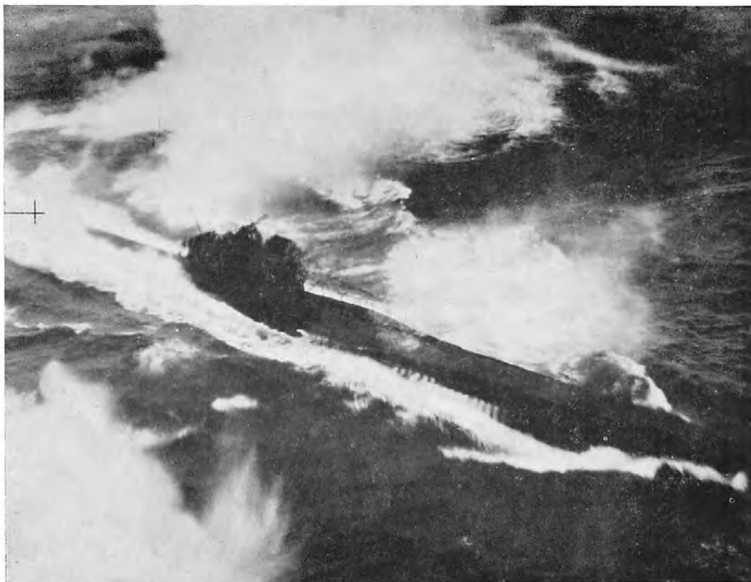
These photographs were taken during the action in which Canso B/162 sank a 500-ton U-Boat on June 11 in northern waters. They are the first photographs which show a schnörkel. The apparatus can be seen lying in its housing forward and slightly to port of the conning tower. A picture of an erected schnörkel in operation is shown on Plate 5.
