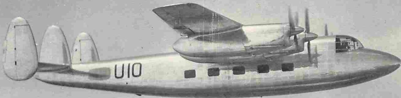
*The Miles Marathon on test flight. On this prototype a central fin has been added to the original design in compliance with ARB requirements. The outboard fins are adjustable longitudinally and it is hoped by this novel means to provide for directional stability on take-off without the necessity for the central fin.*
