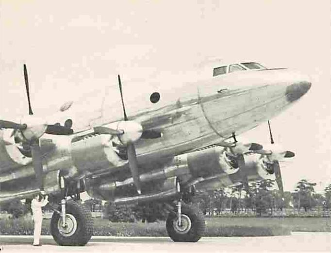
*Rolls Royce Merlin 100 motors in their new circular section cowling*
