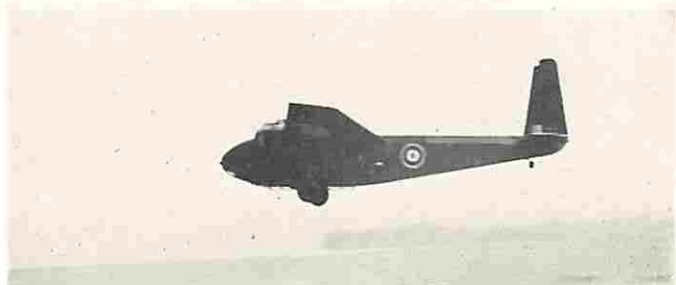
The powered Hamilcar takes off. The Hamilcar is Britain's biggest glider, with a wing-span of 110 ft. and a payload of 17,000 lb. This powered version, the Hamilcar X, will take off under its own power with an all-up weight of 32,000 lb., of which 3,867 lb. is payload. The twin engines are Bristol Mercury XXX. Its original purpose was to extend the range of Halifax-Hamilcar combinations, especially in the Far East
