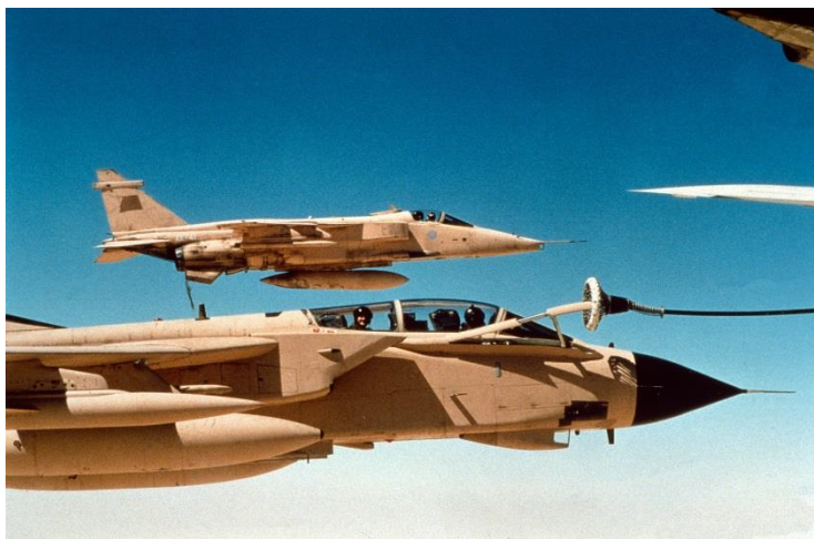
Operation GRANBY: A Tornado GR1 refuels from a VC10 tanker while a Jaguar awaits its turn. Photograph: AHB(RAF)
